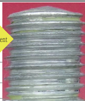
Graph (6) Double Nut (Upper) : Tightening until damage on the bolts threads
