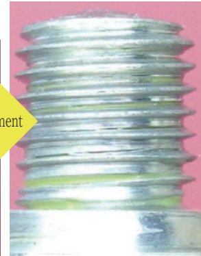
Graph (5) HARDLOCK Convex Nut : Tightening until damage on the bolts threads
