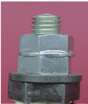
Graph (5) HARDLOCK Convex Nut : Tightening until damage on the bolts threads
