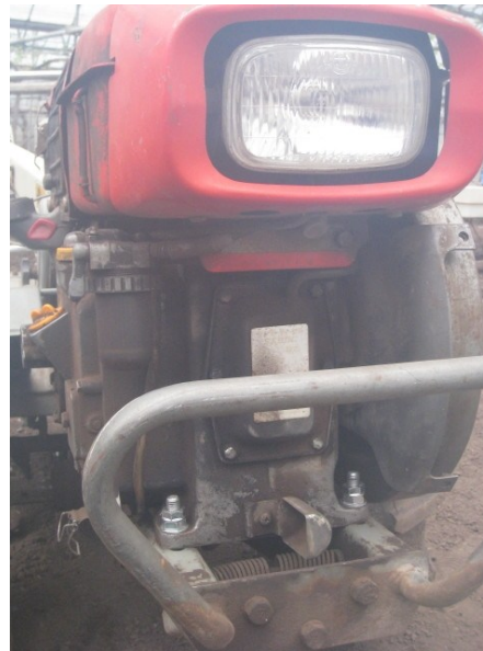
Bumper for Rice planter Engine M12 SUS304
