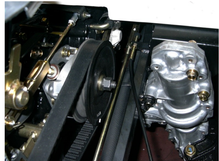
Rice planter Engine counterpulley M12 S45C
