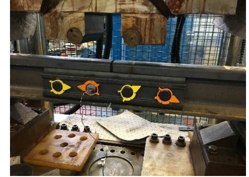
The final testing stage conducted 250,000 cycles over 16 hours
